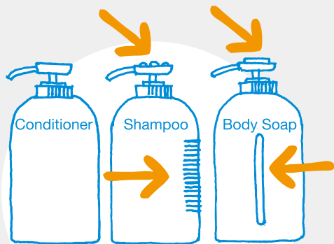
Tactile marks on bottles of shampoo and body soap to distinguish them from bottles of conditioner
